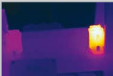
Problem in motor fan bearing
